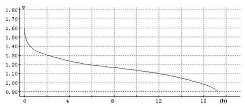
Test Condition: Load Resistor 3.9Ω, 24hrs/day, 20°C±2°C and 60±15%RH
