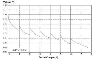
Test Condition: Load Resistor 75 $\Omega$ , 4h/d, 20°C±2°C and 60±15%RH
