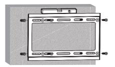
Install the wall plate to the solid wall
