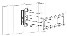
Install the wall plate to the wall
