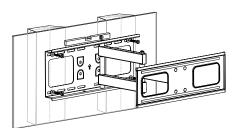
Install the wall plate to the wall
