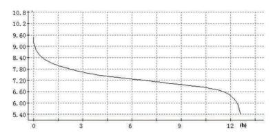
Test Condition: Load Resistor 180Ω, 24h/d, 20°C±2°C and 60±15%RH
